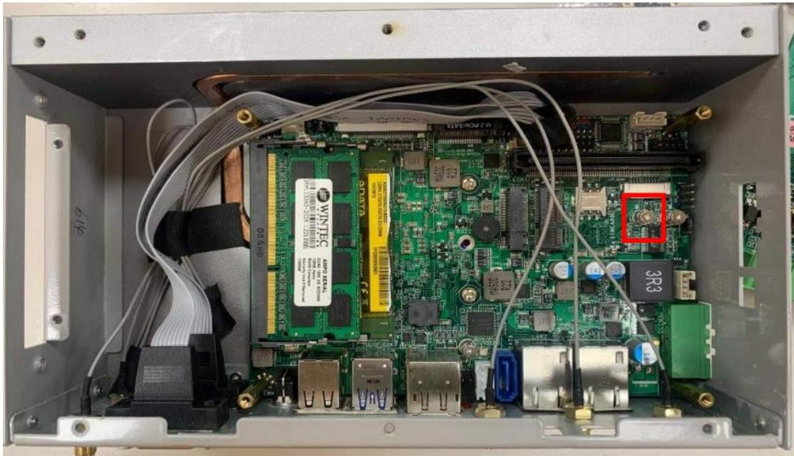
2. Remove the marked screw and use it to lock M2-E-Key and M2 B-Key card to the slot in later installation.
