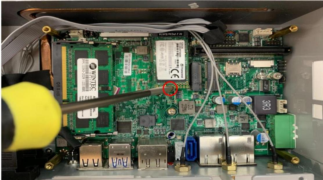
9. Tighten up the screw removed before to the marked spot to secure the card.
