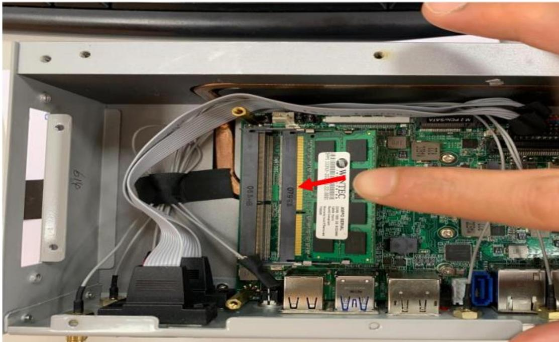
4. Insert the gold-figure side of the compatible SO-DIMM into the slot at a 30 degree angle. See to it that the break of the module fit into the notch of the slot.
