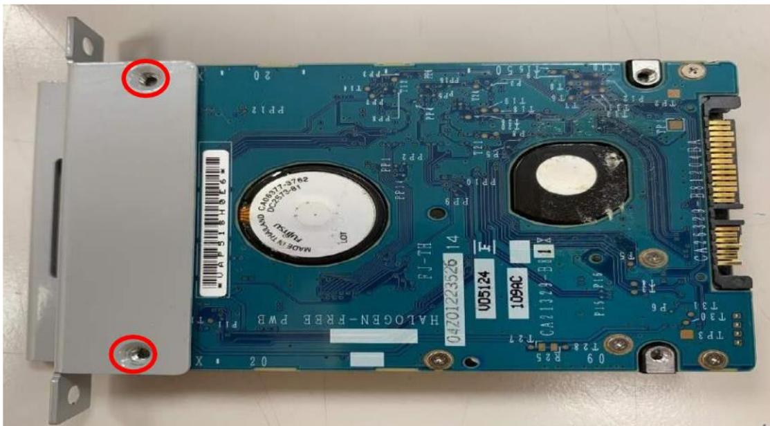
2. Lock the racks with HDD installed by fixing screws to the screw holes marked above.
