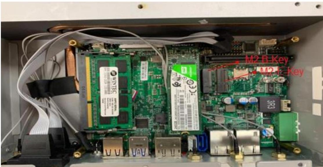
1. Locate the M.2 E (M2E) and M.2 B (M2B) slot on the board.
