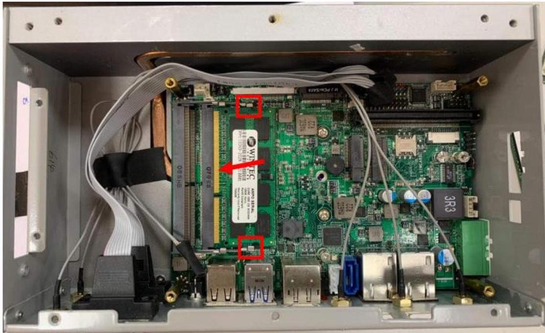
5. And press down to secure the SO-DIMM to the slot. The eject tabs will lock automatically if installing direction is correct.
