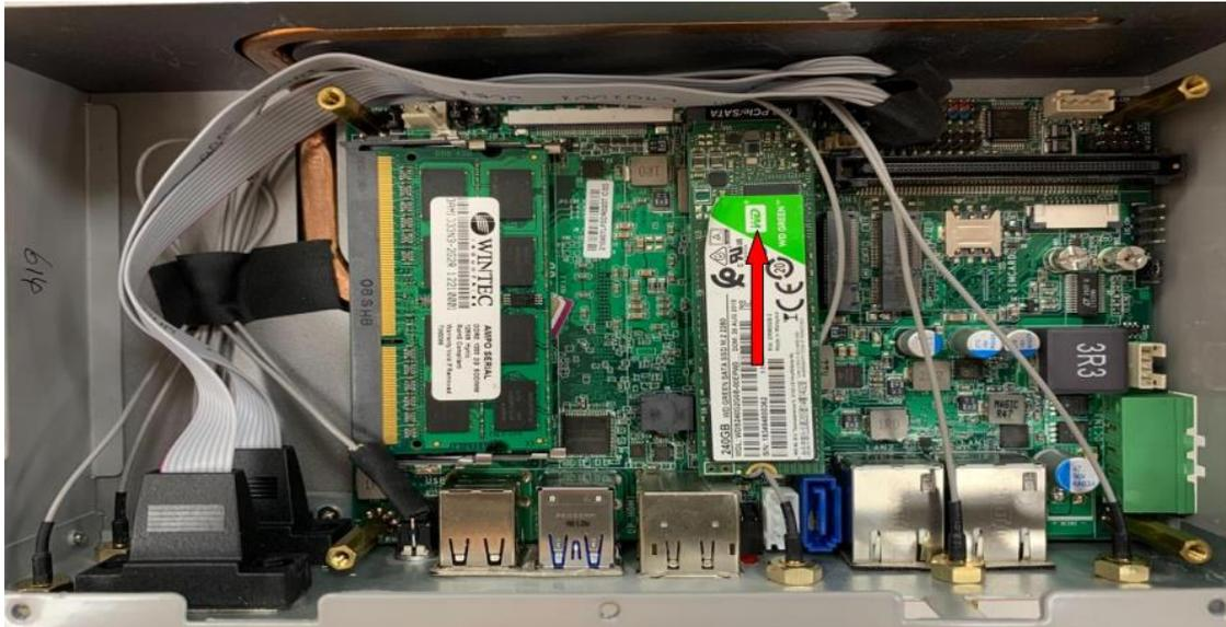
3. Insert the gold-figure side of compatible M.2 M-Key 2280 (PCIe/SATA) card into the slot until the golden finger side fully emerged into the slot.
