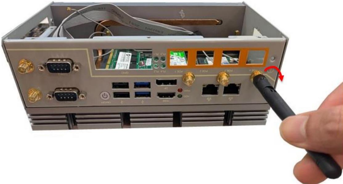
9. The rear panel with antenna screwheads installed.
