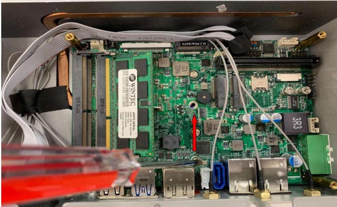
5. For 2242 card installation, please remove the screw and the screw bolt underneath from the default spot MH4 to MH2 at first.
