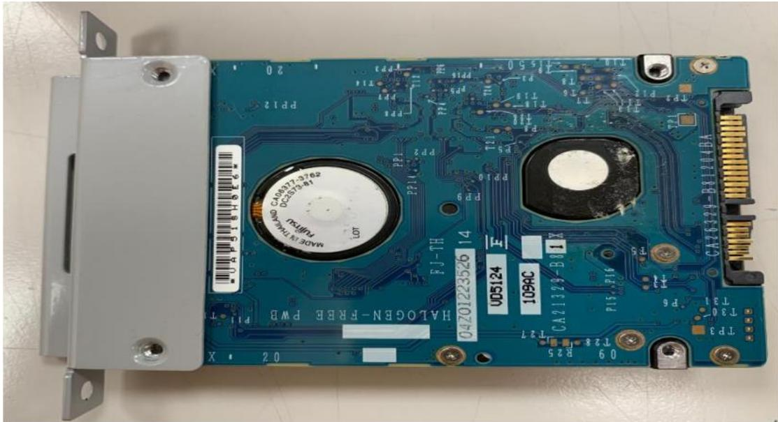
1. User can install up to 2.5" HDD on the tray. Adjust the 2.5" HDD on the tray until the screw holes of the tray matched those in the HDD.
