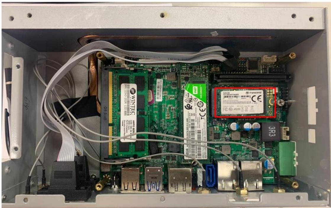
5. Install the compatible card (M2 B-Key 4g/5g) in the same way.
