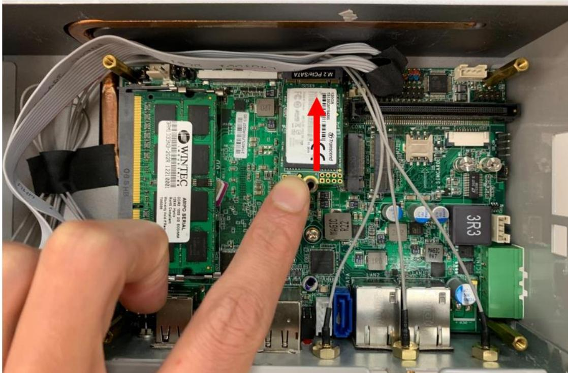
8. Insert compatible 2242 card into the slot.
