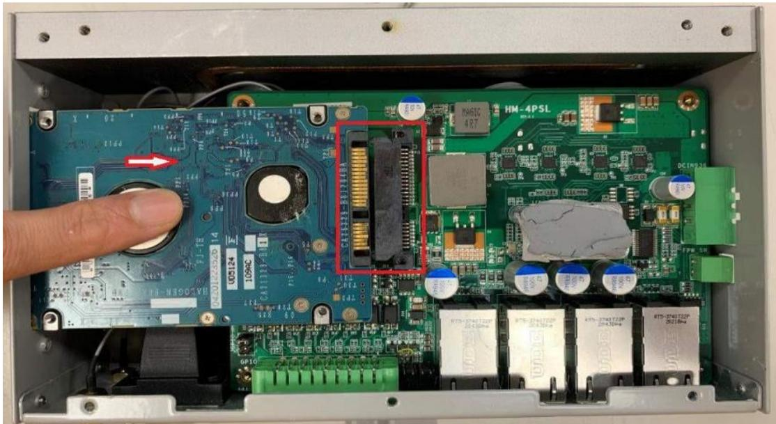
3. Push the interface of HDD into corresponding HDD connector of the board in the direction shown above until it fully fitted into the connector.
