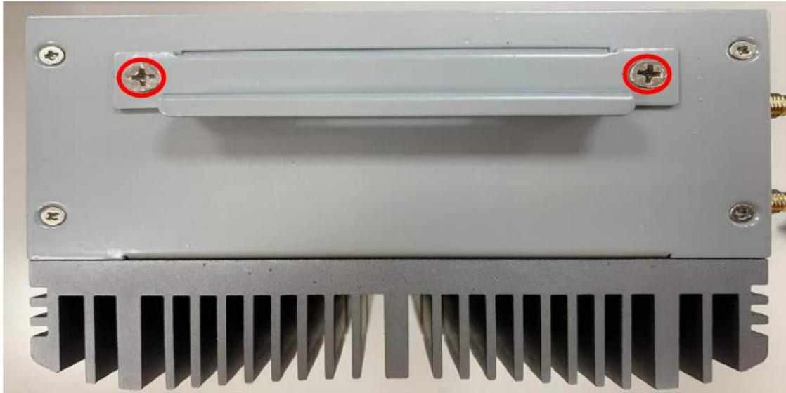
2. Also remove the screws on the side chassis cover that lock the HDD expansion ports.
